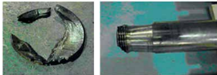
Figure 6: Fragments of the piston rod thread region. Top view of the failed piston rod thread region.
