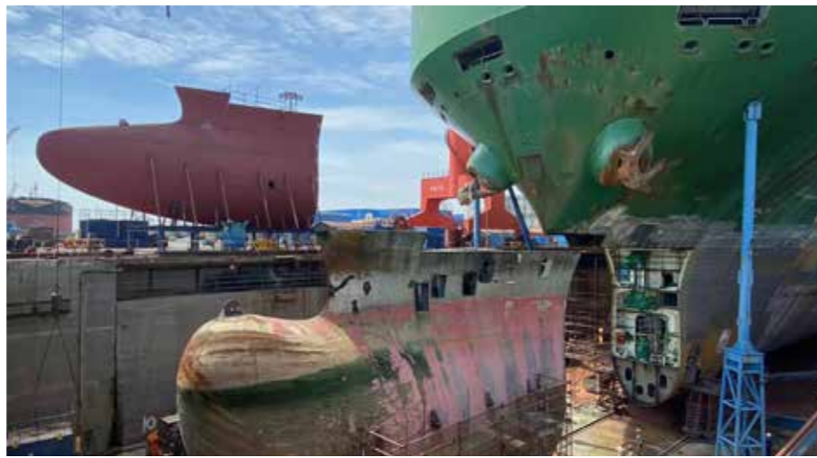
Wallenius Wilhelmsen Precision work at IMC-Yongyue: bow section changeover on a PCTC.
