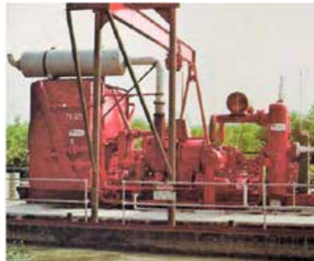
IR2500 rotary engine and RDS-2 reciprocating compressor barge-mounted gas production package in Louisiana, c. 1977.
