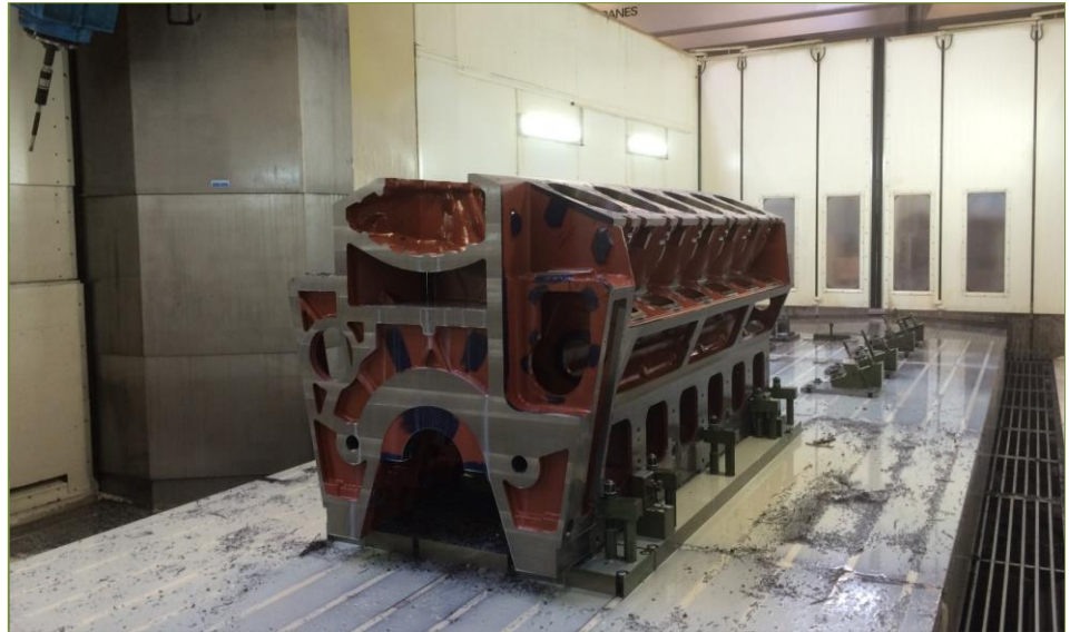
Waldrich milling machine for machining engine blocks up to 40 tons
