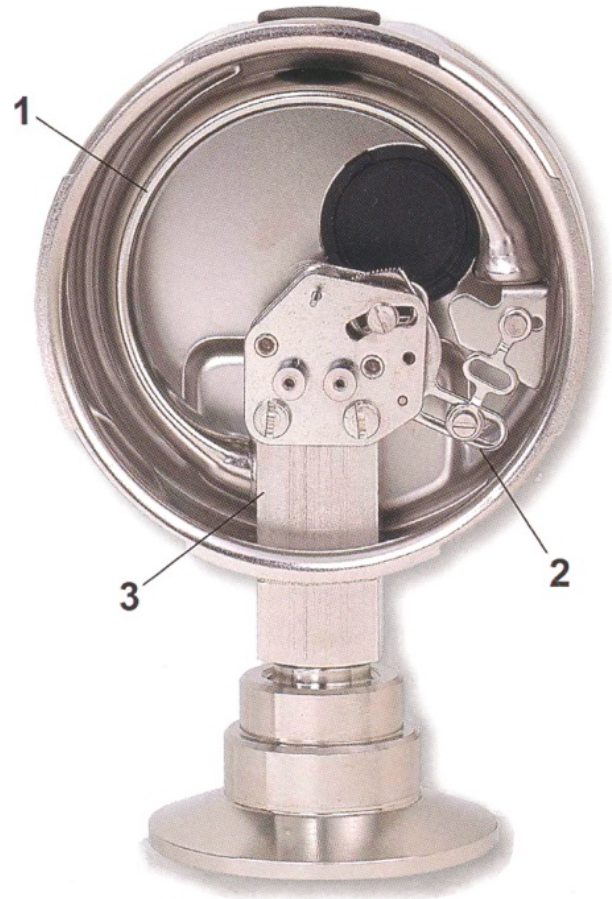
Fig. 2: Bourdon vacuum gauge: 1. Bourdon-tube, 2. lever system, 3. connection tube to connection flange.
