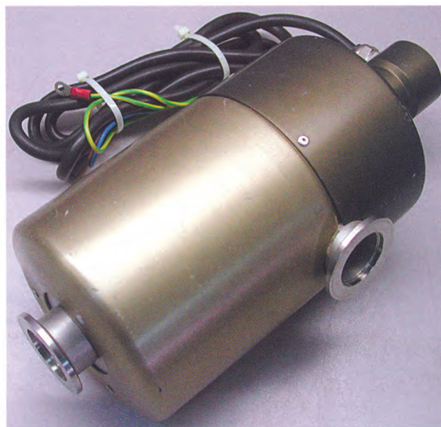
Fig. 3: molecular sieve trap with an electrically operated internal heater to regenerate the trap by heating.
