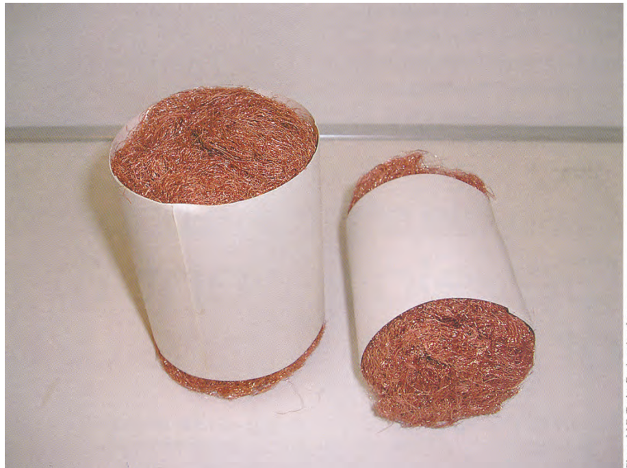
Fig. 4: an in-line adsorbent trap with a disposable copper maze effectively prevents oil from backstreaming towards the upstream vacuum process.
