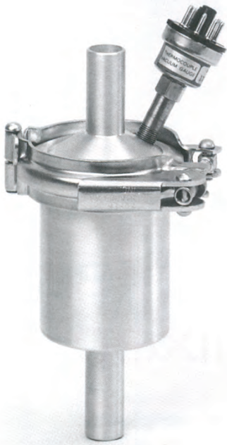
Fig. 4: an in-line adsorbent trap with a disposable copper maze effectively prevents oil from backstreaming towards the upstream vacuum process.
