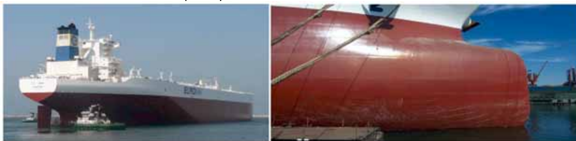
Figure 10. TI Asia newly refurbished with 3rd generation Hydrogel Silicone fouling release technology (left) and after 13 months of sailing between the Arabic Gulf and California at an average speed of 17 knots and estimated activity of 80% (right).
