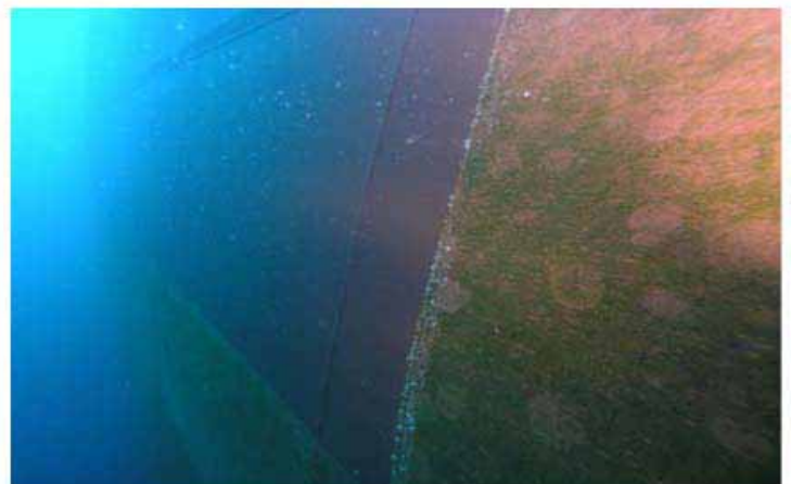
Figure 9. Hydrogel Silicone test patch (left) observed completely free from fouling. Algae and slime observed on self-polishing AF.
